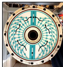
Spacer top-view in the module
